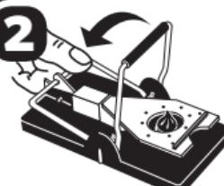
**EASY TO SET:** Place trap in a problem area, preferably near a wall. With trap on a flat surface, pull back slowly on upper bar until it locks firmly in catch. Trap is set when colored bar is in upright position.
