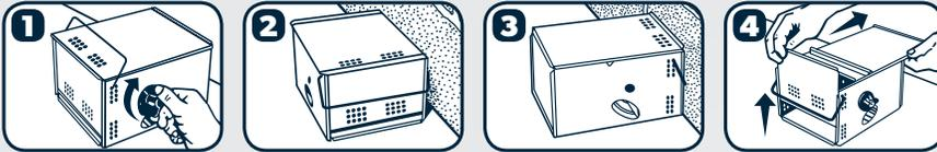
**TO EMPTY:** Simply slide back the top lid and pull up the end plate.
